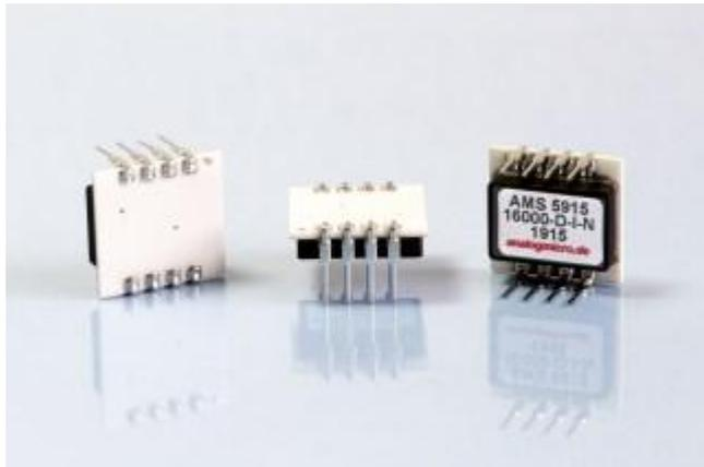
Analog Microelectronics GmbH announces the expansion of its digital board-level pressure sensor series AMS 5915 with I2C output. Now available are special variants for pneumatic applications. These PCB-mountable pressure sensors, made on a robust, thermally insensitive ceramic substrate in a DIP-08 package, are suitable for manifold assembly on flanges with o-ring seals and have a very low assembly height of approximately 4 mm.
