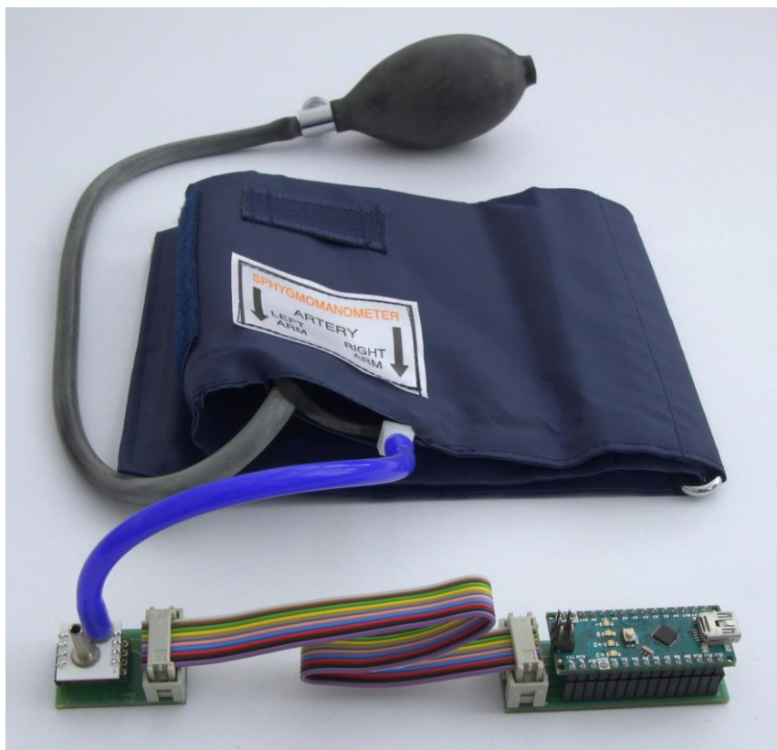
Figure 1: Measurement setup using an AMS 5915, Arduino Nano, the AMS 5915 Arduino Nano kit [4] and an inflatable cuff
