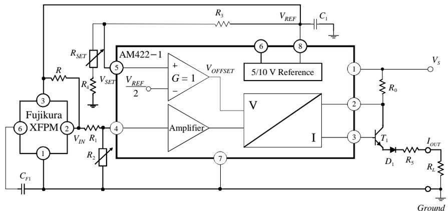
Figure 2: the application needs few external components
