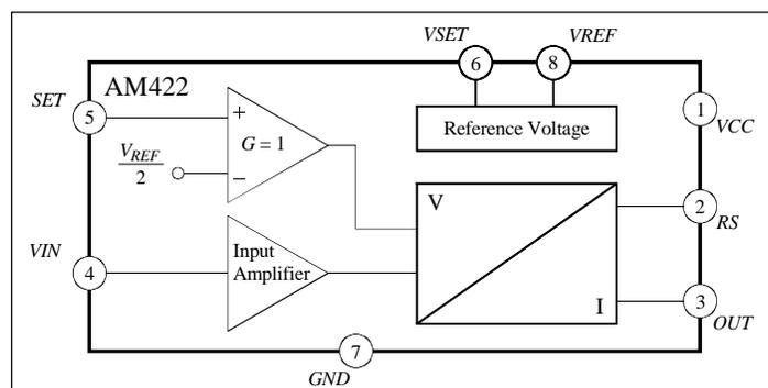
**Figure 1:** block diagram of the voltage-to-current transmitter AM422
